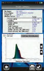
The all new Cell QC app allows you to run multiple tests of the same sample type in Batch Mode. User-to-user variability is eliminated by auto-finding both live and dead cell populations, while exlcuding cellular debris and RBC contamination (PBMC app). Batch mode data is exported in CSV and FCS 3.1 formats
