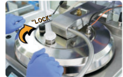
Safety lock with 12 hooks !
